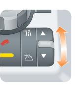
**HIGH** range should be used for all normal road driving and also for off-road driving across dry level terrain.
